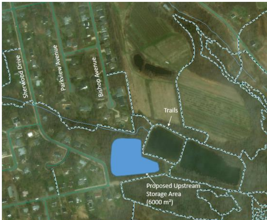
Figure 8.18: Proposed Stormwater Storage Area in Open Space west of the Reservoir near Pleasant Street
